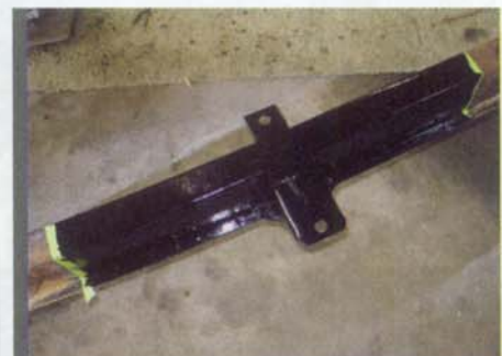
With three even coats of RustSeal applied, the framerail was looking better than new. The test area was done using a brush. However, once a few future modifications are finished, the entire chassis will be done using an HVLP spray gun.
